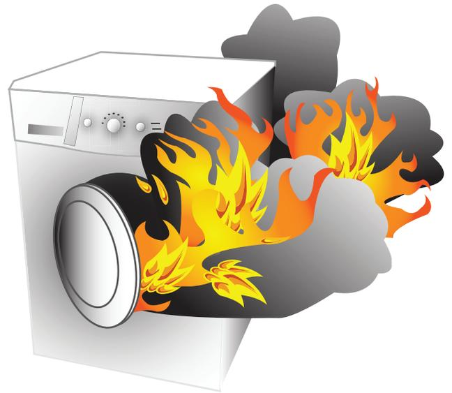
If clothing is damp at the end of a typical drying cycle or drying requires longer times than normal, this may be a sign that the lint screen or the exhaust duct is blocked. Check the outside dryer vent while the dryer is operating to make sure air is escaping. If it is not, exhaust duct may be blocked. Discontinue use of dryer and call a qualified service person to check the appliance and ductwork.
